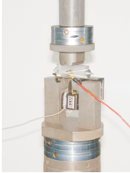
Figure 13: Four-point-bending test fixture with acoustic emission transducer and crack opening displacement gage (PMMA specimen).
