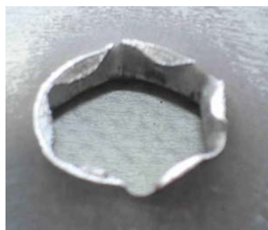
Figure 3: Plastification at the corner of the bolt and sudden fracture along the side of the bolt
