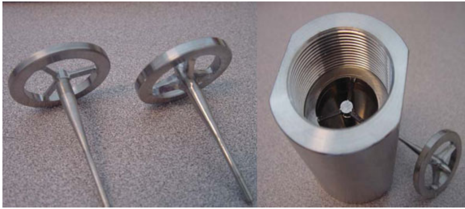
FIG. 1. A picture of the annular die showing the various inserts that are used to change the gap. [Color figure can be viewed in the online issue, which is available at www.interscience.wiley.com .]
