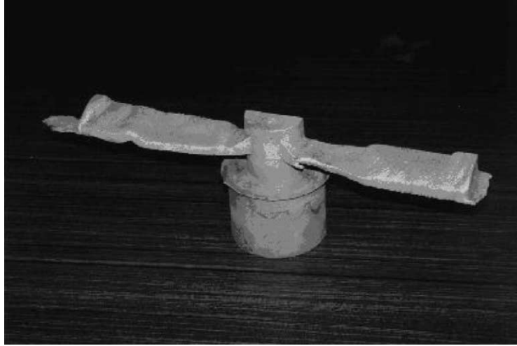
Fig. 1. Flow instability in SSMP: toothpaste behavior. Filling from the center towards the arms (Courtesy of Aluminium Pechiney).
